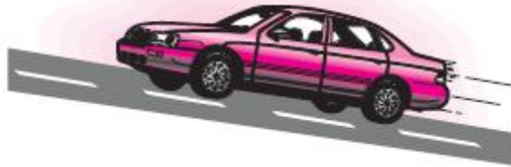
Fig. The macroscopic energy of an object changes with velocity and elevation.
